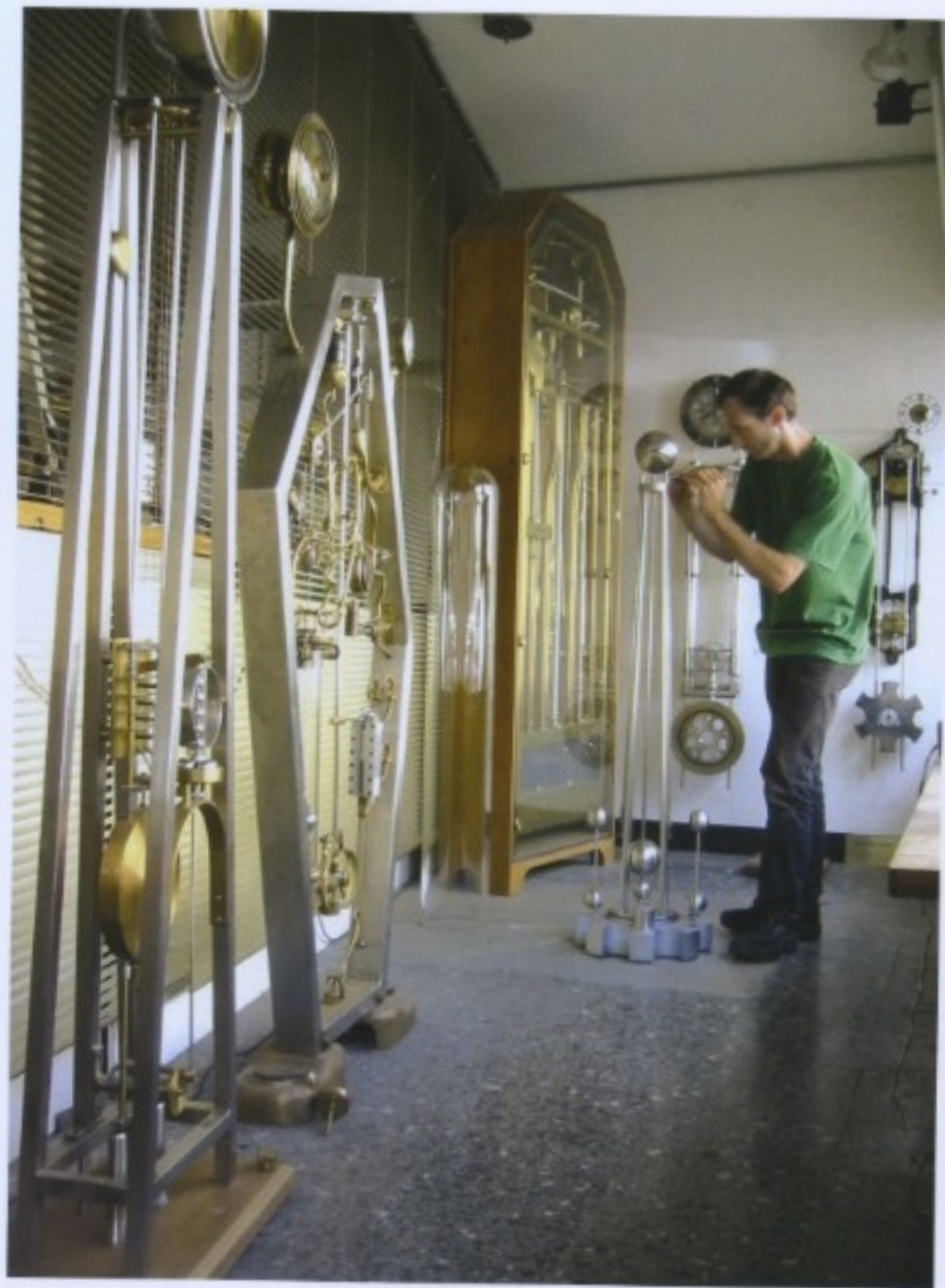
Betrisey adjusts his clock with the vacuum chamber removed. The 33-pound glass bell sits to the clock's left and was the most expensive part at $1,000. Its 0.4-inch walls keep a near-perfect vacuum inside so that only light rays push the pendulum.
